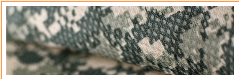
3D spacer fabrics offer innovative solutions with excellent breathability, various elongation, and stability. A 3D spacer fabric comprises three integrated layers: two outside layers attached to a layer of vertical filler yarns to provide varying levels of thickness for volume, resilience, and cushioning.
